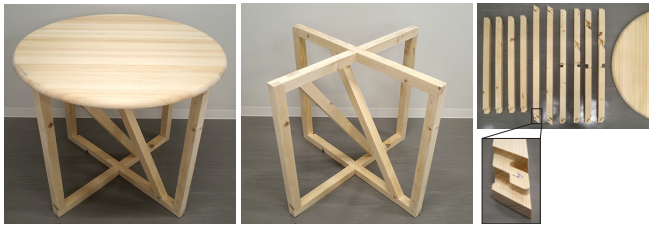
Figure 21. Table fabricated from 10 timbers connected by 14 nail-free and glue-free joints including four oblique ones.
