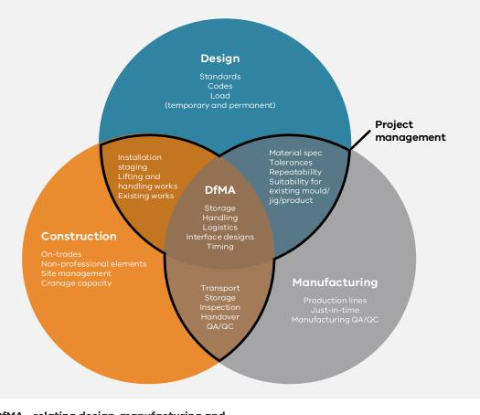
DfMA - relating design, manufacturing and construction management of OSC
