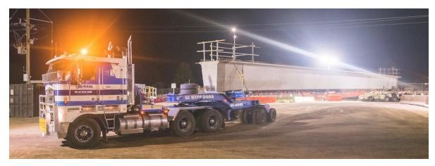
Large precast beam delivery with rear dolly requiring clear swept path [Credit Westkon]
