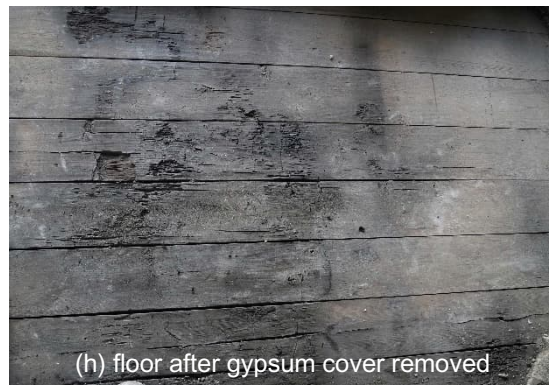
Figure 25. Photographs of Bay 1, Bay 2 and Bay 3 near or after the end of Test 5.
