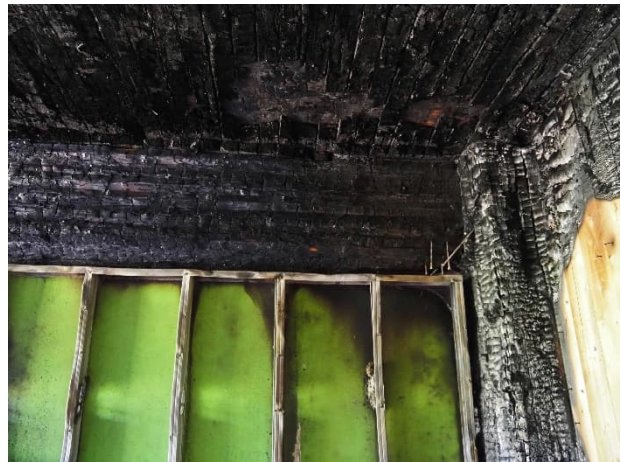
Figure 43. Charring and temperatures in ceiling-beam-column connection in Test 2.
