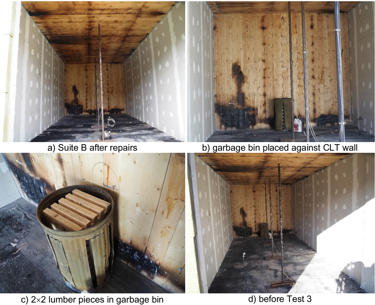
Figure 64. Simulated construction site with garbage bin (before Test 3).
