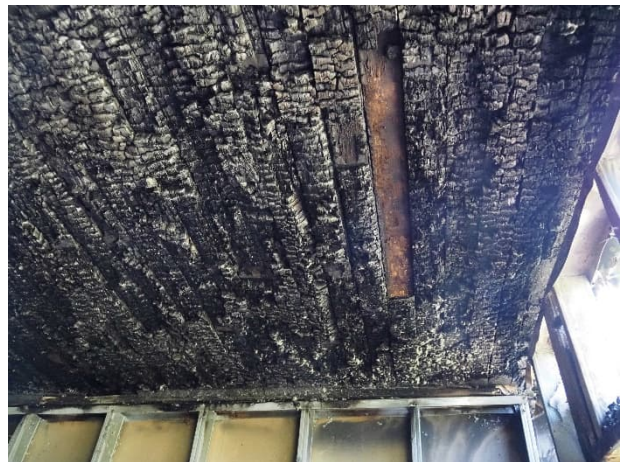
Figure 44. Some delamination from CLT ceiling in Test 2.
