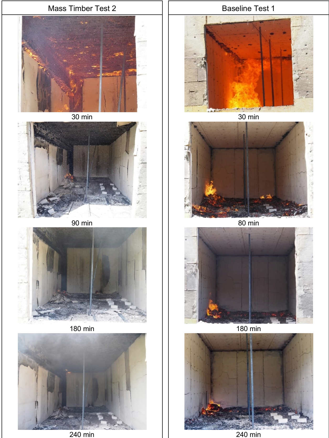
Figure 36. Comparing Test 2 with Test 1 – Decay stage of the fire.
