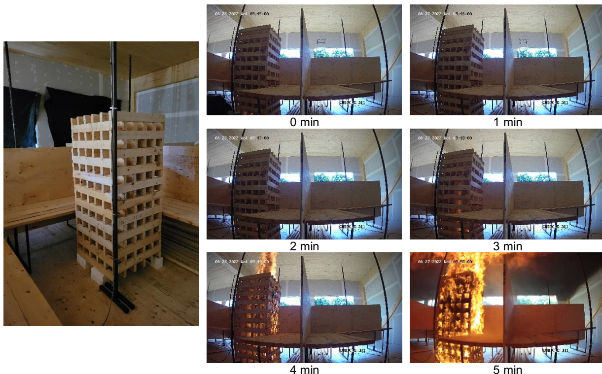
Figure 7. Ignition of wood crib in Cubicle 3 (adjacent to Cubicle 1) for Test 5.
