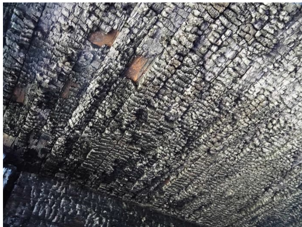
Figure 44. Some delamination from CLT ceiling in Test 2.
