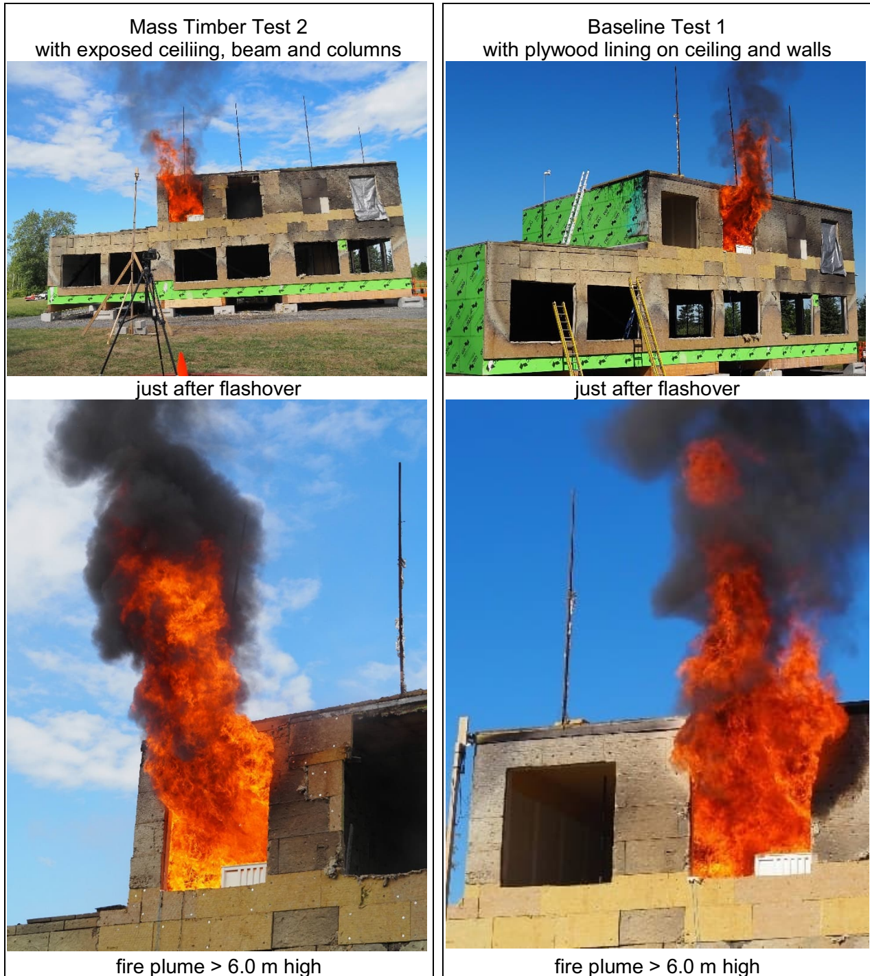
Figure 45. Comparing Test 2 with Test 1 – Fire plumes issued from openings.
