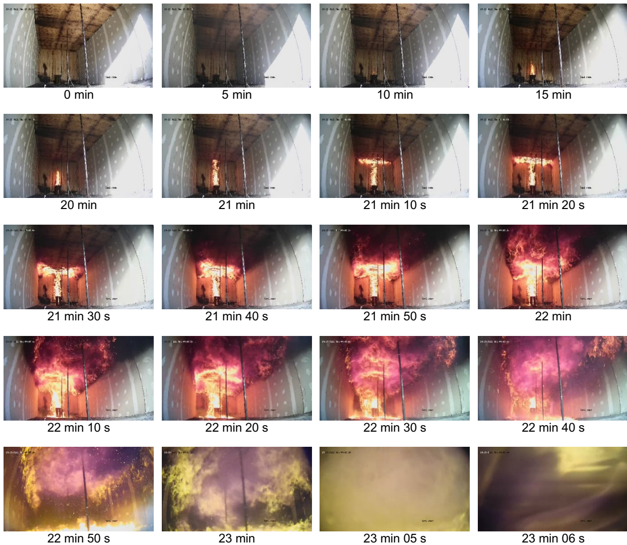
Figure 65. Initial fire development in Test 3 (interior view).
