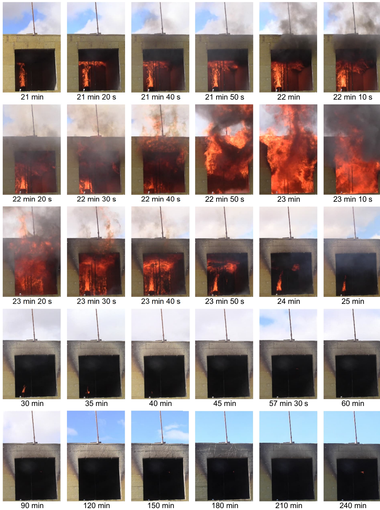
Figure 66. Fire development in Test 3 (exterior view).
