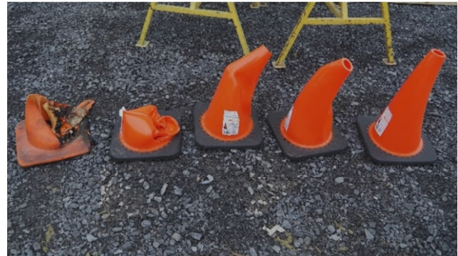
Damaged plastic safety cones (from left to right) which were placed at 11, 14, 17, 21 and 24 m away.
