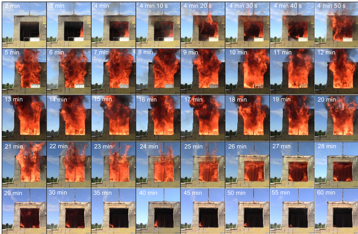
Figure 35. Exterior view of fire development during mass timber Test 2.
