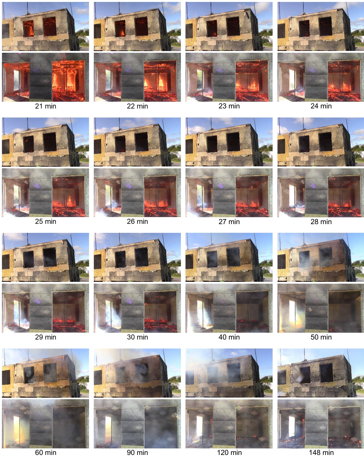
Figure 51. Views from exterior and through two northern openings in Test 4. (Continued from previous page)
